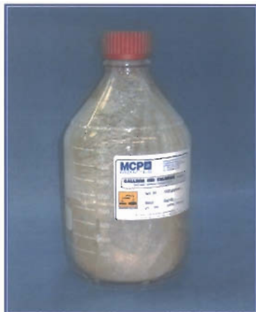
Anhydrous gallium trichloride packed in a 2 litre borosilicate glass bottle with pfe insert in screw cap
